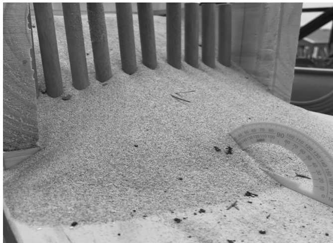
Figure 3. Experiment undertaken on dry beach sand showing failure will occur through the soldier piles at the angle of repose
