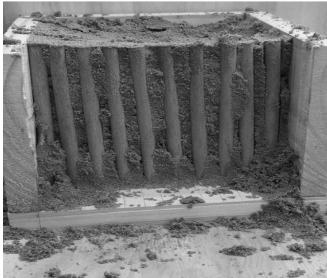
Figure 2. Experiment undertaken on moist beach sand illustrating the effect of capillary cohesion.
